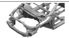
The ACE Body Structure with its front-mounted polygonal main frame is designed to prevent structural penetration while distributing forces evenly through multiple major load bearing pathways
