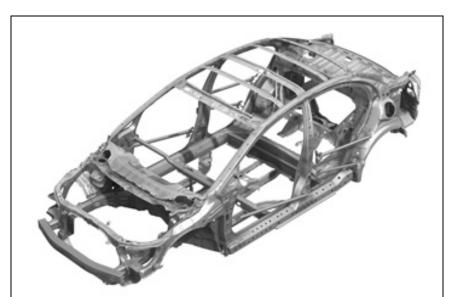
A new body design with the ACE Body Structure and extensive use of high strength steel create a new generation platform that is safer and stronger
