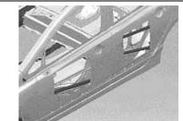
Civic doors feature high strength steel side impact protection beams
